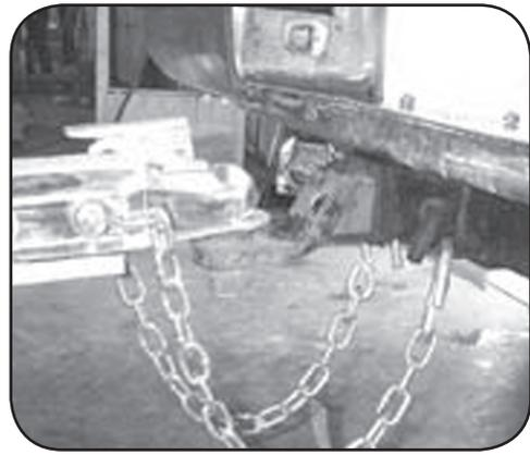
Check that trailer safety chains are properly connected. Check that all trailer lighting is hooked up and working correctly.
