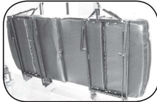
This is the bed position. To continue on to the dinette set-up, pull up on the head of the bench and it will 'jack-knife' into place.
