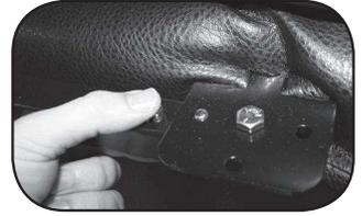
Be sure each leg is fully extended and locked in place.
