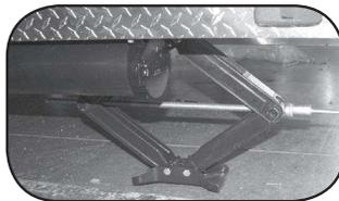
For best results, crank the tongue jack down to a lower position than the rear of the unit. In this position drop the rear jacks. After you have locked the rear jacks into place go back to the tongue jack and crank up until it is a little higher than the rear. Repeat jack procedure on front jacks.
