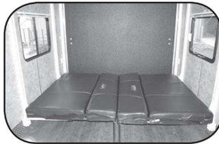
Fold the seat-backs up and over each bench. Once the bed or seats are in the desired position, re-engage the HappiJac brake.
