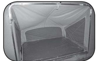
Lock the bent end of the bimini pole into the bracket above the bunk opening.
