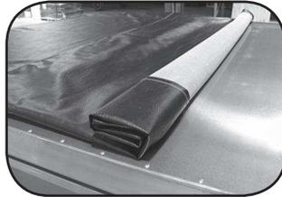
**Store:** After rolling the tonneau cover, attach it to the front of the unit with the two straps provided. They hold the cover in place while camping.
