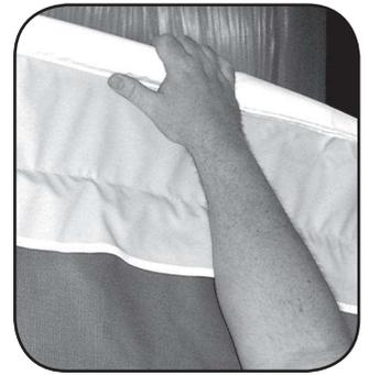
Fold the edges of the bunk side tent under the bunk where the Velcro will adhere and gently pull the bungee cord over the small posts located on the underside of the bunk.
