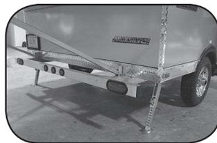
For best results, crank the tongue jack down to a lower position than the rear of the unit. In this position drop the rear jacks. The jacks are spring-
