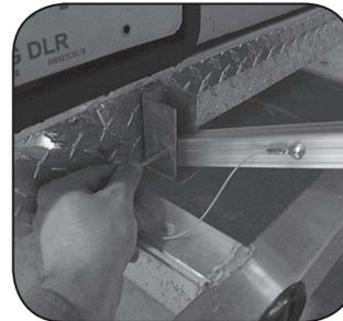
When all four poles are in place and the cotter pins are completely through (bracket, pole, bracket), you're ready to open the unit.
