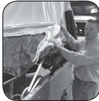
**NOTE:** Before you snap the tent into place, go to the door where you will find a center separation pole. Snap it on between the two center bimini poles. This will provide additional strength and support in the center of the tent. Once this is done, you can proceed outside again, snapping the tent to the perimeter of the camper and attaching the Velcro bunk ends and bungees around the unit.
